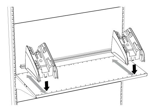
Once the correct depth has been determined, remove the tape and fix the profile to the shelf
